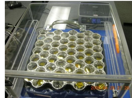
QZS-1GPS 35, 56 * 40.6 mm cubes TIR Cubes 32K – 40K Km orbit 45 deg inclination
