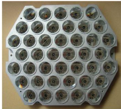
COMPASS M1 42 * 33 mm cubes TIR Cubes 21,500 km orbit 55 deg inclination
