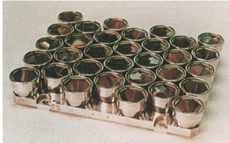
GPS 35, 36 32 * 36 mm cubes Al Coated Cubes 20,000 km orbit 50 deg inclination
